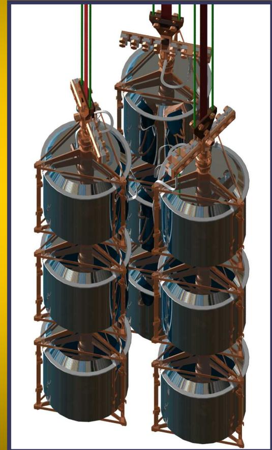
GERDA PHASE I detectors mounted vertically into strings in low-mass Cu support operated in LAr/LN<sub>2</sub>
