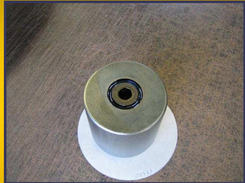
Prototype diode (total mass 1.6 kg) refurbished by CANBERRA using the same technology as for the enriched diodes. The FWHM in a test cryostat is 2.2 keV at 1.332 MeV.
