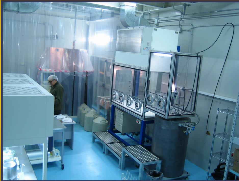
Detector test bench, Rn 'free bench' and clean bench. Ar level is monitored by weighting cells, Rn by Lucas cell (10 Bq/m<sup>3</sup>) and humidity is kept low (30%).
