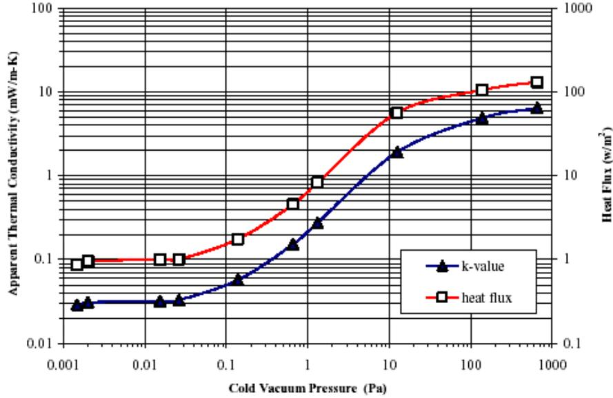
Figure 11: Variation of heat flux (right scale) and apparent thermal conductivity in a MLI blanket (30 layers, 7 mm total thickness) with cold vacuum pressure [Fes 02].
