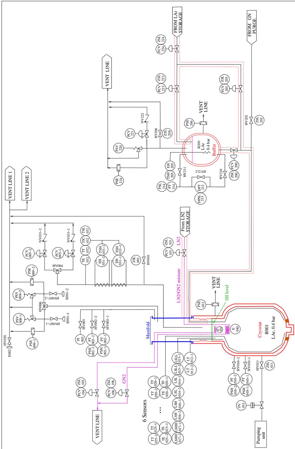
Figure 13: Piping and instrumentation drawing (PID) for the cryogenic infrastructure.
