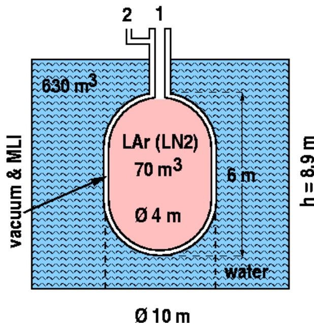
Figure 15: Vessel dimensions assumed for discussion of safety aspects. (1) indicates the neck of the vessel, (2) the tube through which the space between inner and outer container is pumped. Within this space the multilayer insulation (MLI) is mounted.
