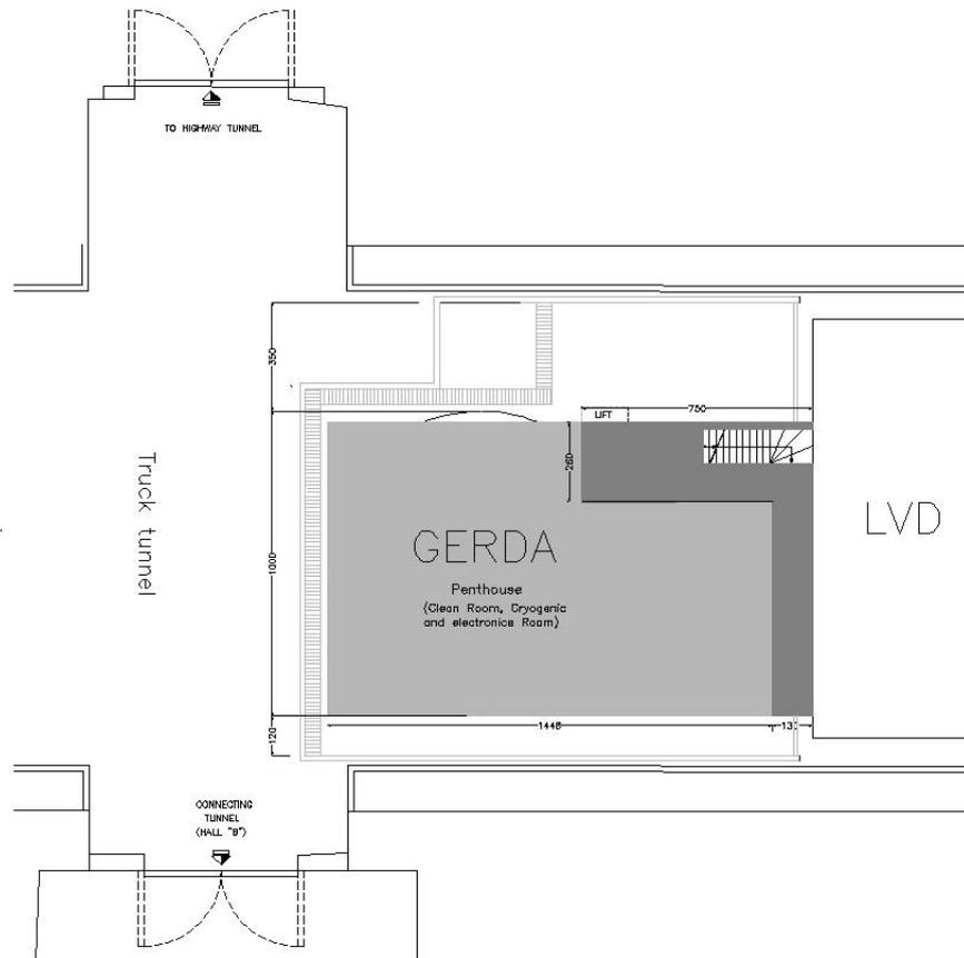
Figure 2: Layout of the Main Experimental Site of GERDA in Hall A (dimensions in cm).
