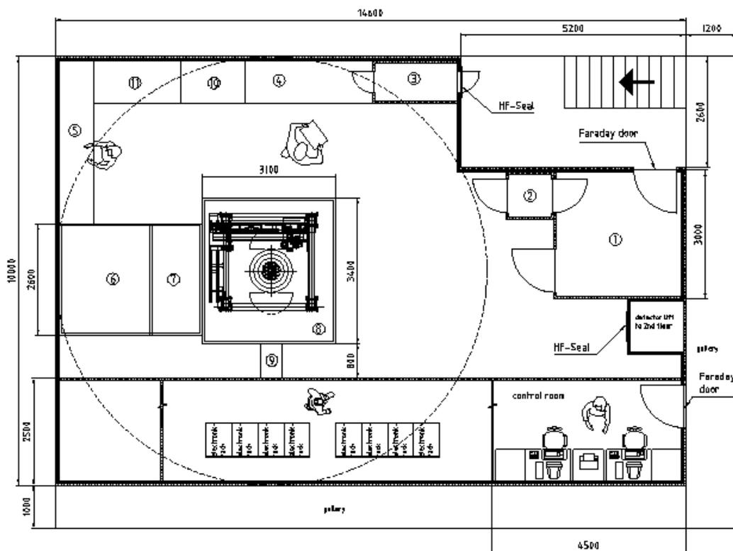
Figure 14: Layout of the penthouse [int.ver. 8] on top of the vessel with clean-room, lock system and the electronics-room. Numbered components are specified in subsection 6.3.
