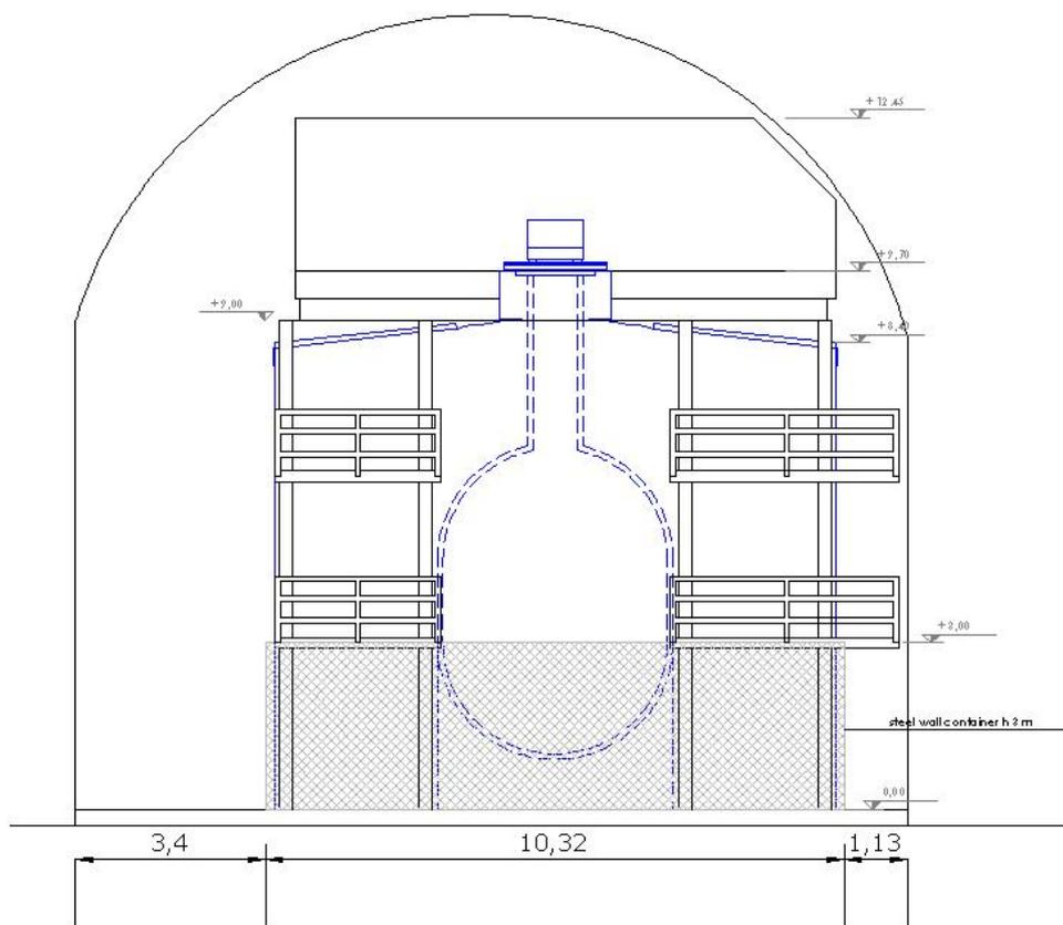
Figure 4: View of GERDA cross section from TIR tunnel.
