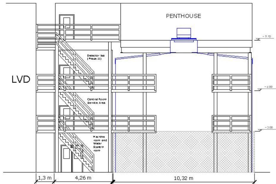
Figure 7: Plan of water vessel and laboratory building: lateral view
