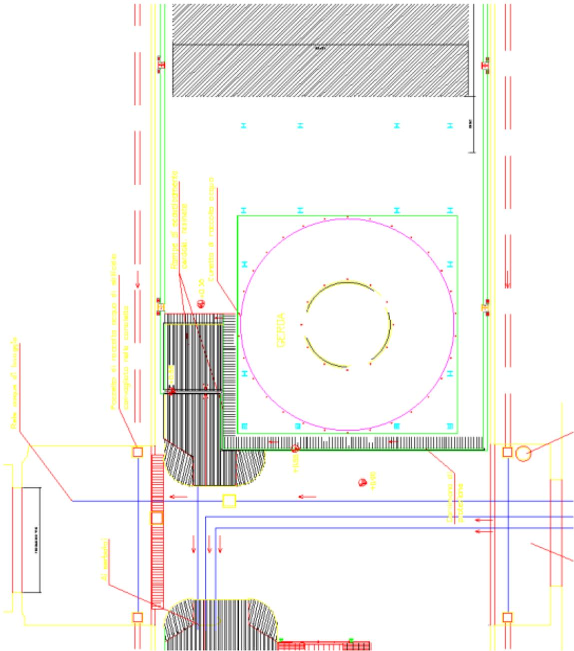
Figure 9: The pipe system devoted to drain the water tank, running below the TIR tunnel.
