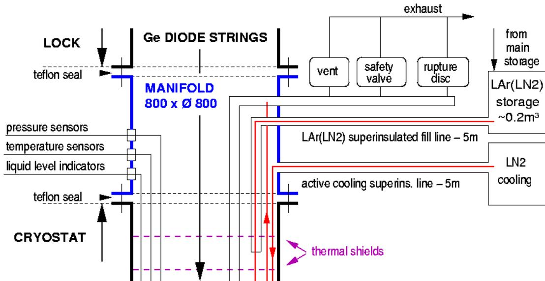
Figure 12: Schematic of the manifold through which indicated devices penetrate into the cold volume.
