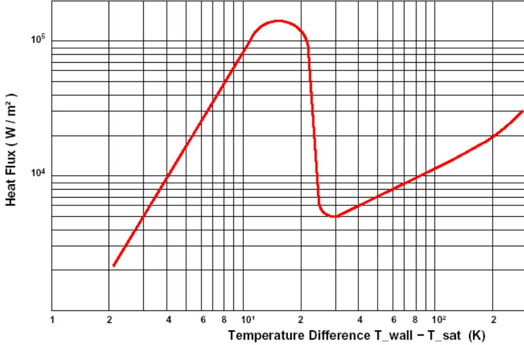
Figure 17: Pool boiling heat transfer characteristics of LN<sub>2</sub> at atmospheric pressure (from [Van 63]).
