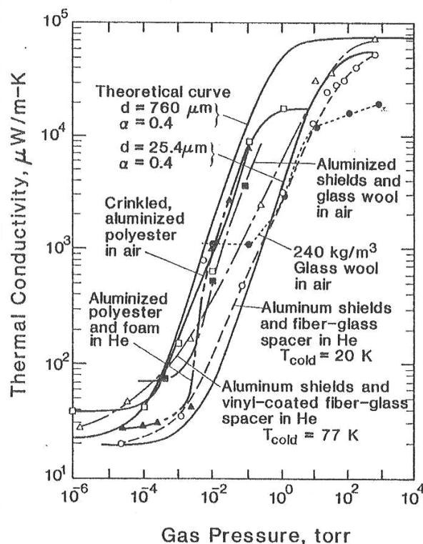
Figure 16: Thermal conductivity of superinsulation in dependence of gas pressure [Tim 89].
