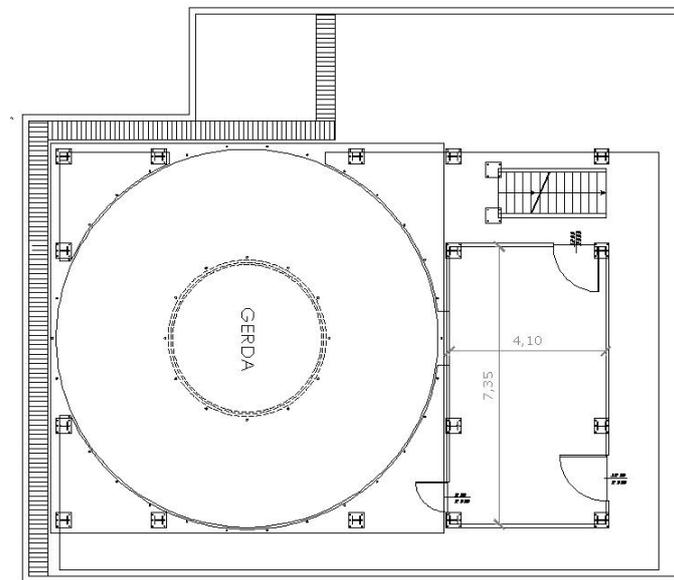
Figure 5: Plan of water vessel and laboratory building: ground and first floor
