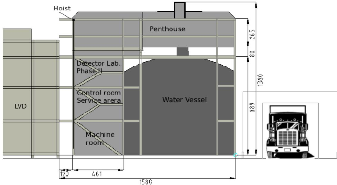
Figure 3: OLD (to be replaced) Lateral view of the GERDA experiment in Hall A (dimensions in cm).
