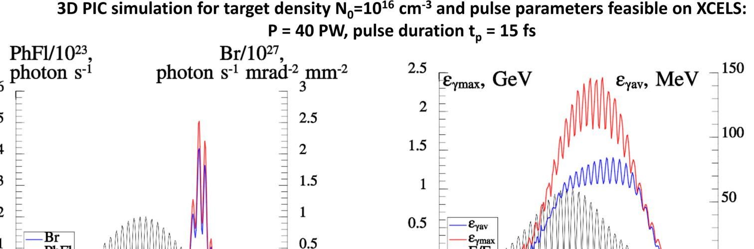
Dash-dotted line – spectra without cascade, solid line – spectra with cascade, (in the inset) dotted line – difference between these spectra, maximum corresponds to maximum probability of photon decay Cascade increases number of high energy photon for power < 30 PW and decreases it for power > 30 PW
