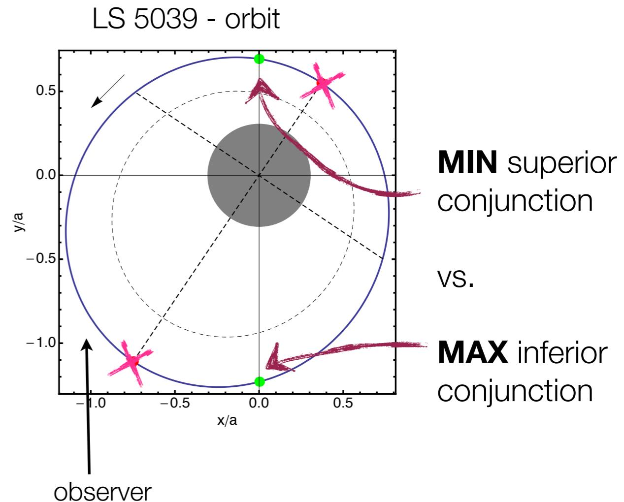
For X-ray point source at compact object, absorption effects can be seen only around superior conjunction.
