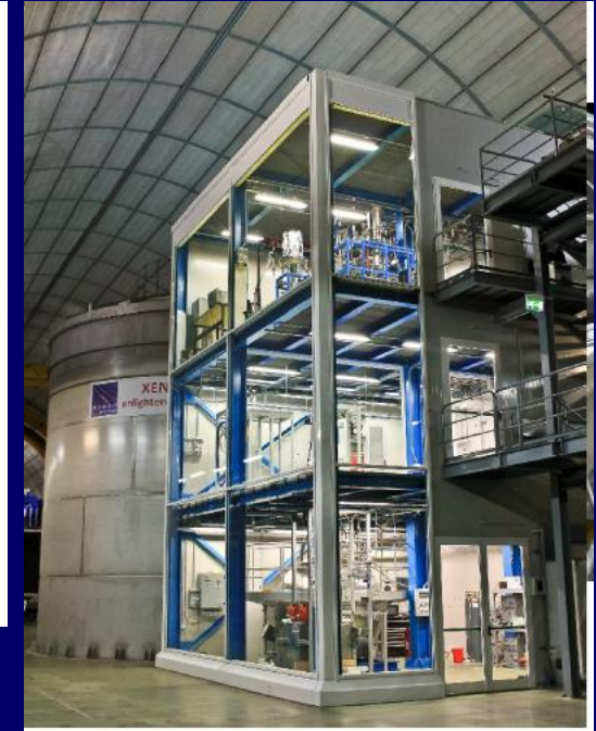
XENON1T (XENONnT) 2012 - 1000 cm drift TPC 3300 (7000) kg xenon \sigma_{SI} < 1.2 \cdot 10^{-47} \text{ cm}^2 ( < 2 \cdot 10^{-48} \text{ cm}^2 )
