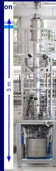
XENON100 2008 - 2015 30 cm drift TPC 161 kg xenon \sigma_{SI} < 2.0 \cdot 10^{-45} \text{ cm}^2
