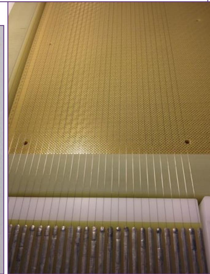
distance between LEM & anode should be kept constant since it affects the gain. Here we had one module surveyed at the metrology lab. Planarity is within ~100 microns which is very acceptable in terms of gain variation (< 5 %).
