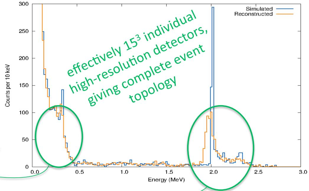
Reconstruction of a typical 2 MeV positron event.
