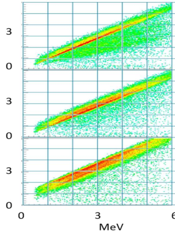
(left) reconstructed response to 2 MeV positrons; (*right*) response to a reactor neutrino spectrum (with statistics reflecting only a one-day exposure).
