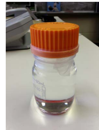
LAB+surfactant+H 2 O+ \text{natTe} +wavelength shifter
