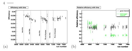
**Fig. 4.** (a) Collection efficiency of Cherenkov light from muon analysis with time. Some hardware changes are indicated. The run numbers are from October to December 2002. (b) Monitoring of the relative efficiencies of two channels.
