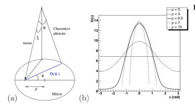
Fig. 2. (a) Geometry of the Cherenkov emission from a muon near the mirror:  $\xi$  is the inclination of the muon to the vertical,  $\rho$ the impact parameter, and  $\theta$  the Cherenkov angle. (b)  $D(\phi)$  for different impact parameters.
