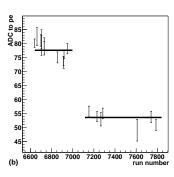
Fig. 1. (a) Example of gain determination in high gain channel. (b) Gain of one damaged pixel with run number; the gain decrease is due to a too bright illumination.
