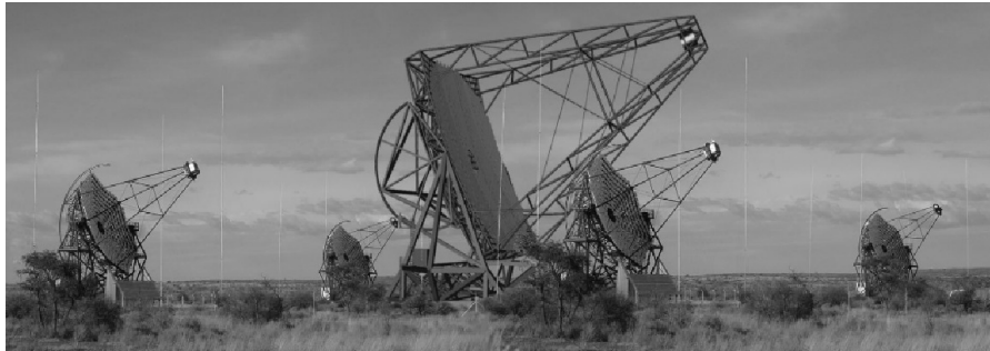
Figure 1: Photo of the current four-telescope H.E.S.S. Phase-I array, with an artist's impression of the Phase-II 28m \varnothing telescope (VLCT) in the centre of the array superimposed.
