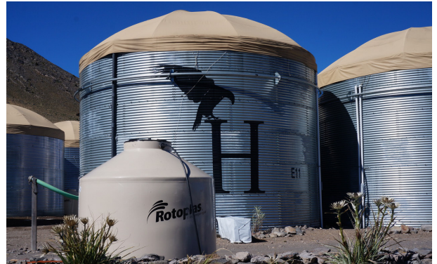
An “outrigger” tank in front of the main detector array of HAWC in Mexico.
