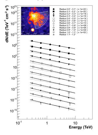
Fig. 8 Energy-dependent VHE morphology of pulsar wind nebula HESS J1825-137, showing a softening of the spectra with increasing distance from the pulsar. The plot shows the energy spectra in radial bins as indicated in the inset (with the dashed line from the innermost region for comparison). From Ref. [82]
