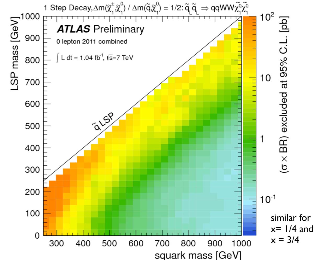
Exclusion limits in the squark-LSP mass plane for direct [left] and one-step [right] squark decays.
