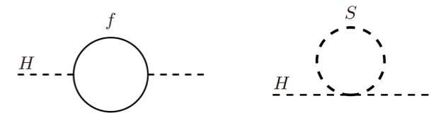
$$\begin{aligned}\delta m_H^2 &= \left(\frac{g_f^2}{16\pi^2}\right) (\Lambda^2 + m_f^2) - \left(\frac{g_S^2}{16\pi^2}\right) (\Lambda^2 + m_S^2) \\ &= \mathcal{O}\left(\frac{\alpha}{4\pi}\right) |m_S^2 - m_f^2|\end{aligned}$$
