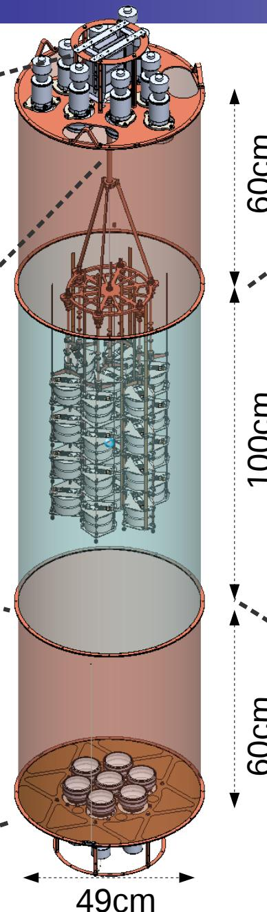
810 scintillating fibers coupled to SiPMs
