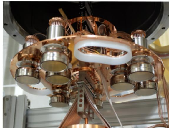
Cu cylinder with wavelength shifting reflector foil
