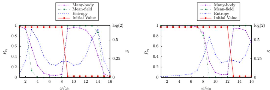
**Figure:** Initial and final neutrino spectra, along with the respective final state entanglement entropies, for the evolution of initial states  $|\nu_e\rangle^{\otimes 8} |\nu_x\rangle^{\otimes 8}$  (left) and  $|\nu_e\rangle^{\otimes 12} |\nu_x\rangle^{\otimes 4}$  (right).
