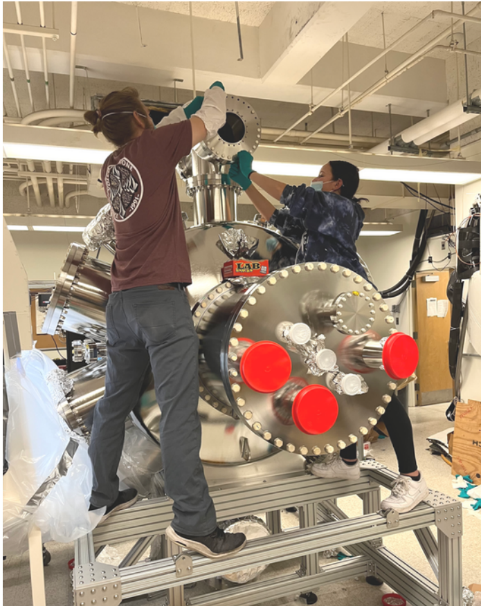
Vacuum vessel- now at 1e-7 mbar
