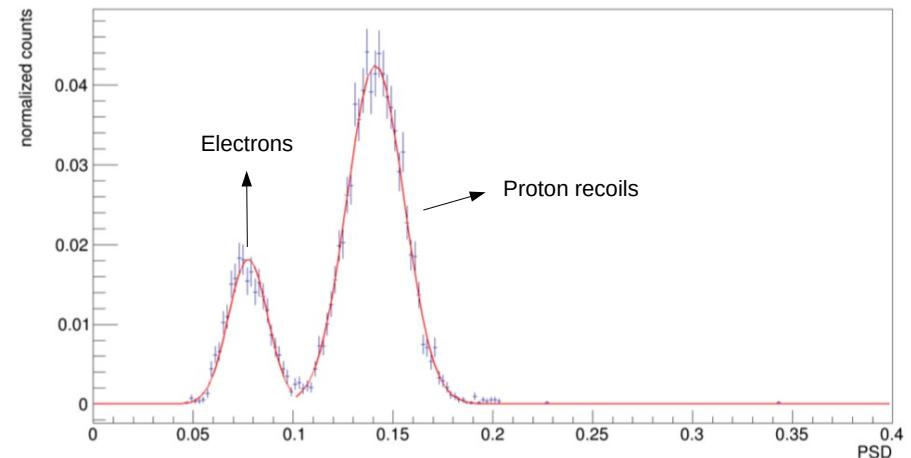
$$\text{PSD} := \frac{Q_{\text{tail}}}{Q_{\text{tot}}}$$
