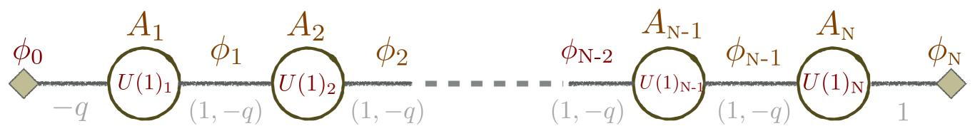
Each site has a  $U(1)_i$  gauge symmetry with  $A_i^{\mu}$  gauge boson. Complex scalar fields  $\phi_i$  are the link fields.
