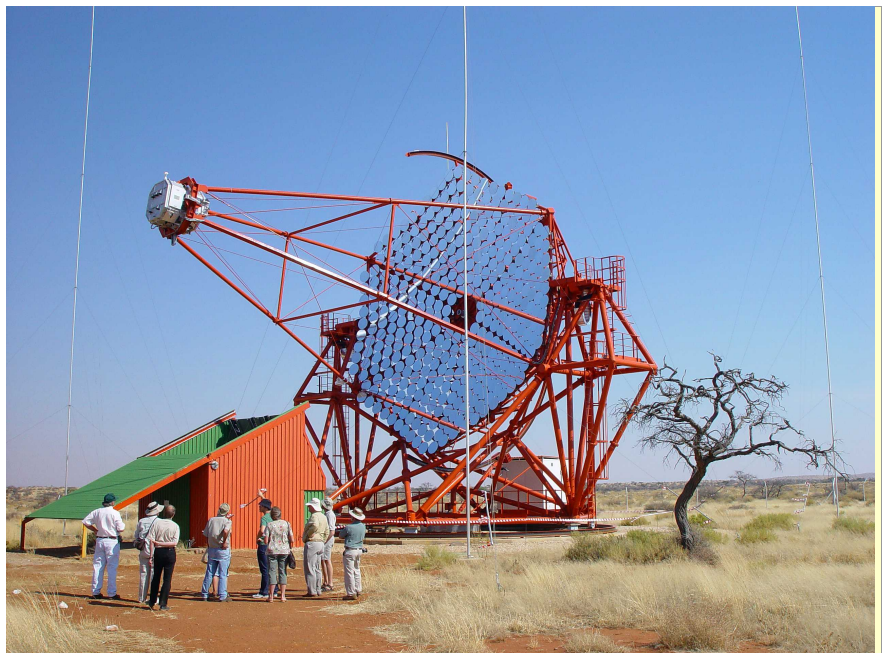
H.E.S.S. Telescopes : The four identical telescopes of the High Energy Stereoscopic System in Namibia detect faint atmospheric flashes caused by the absorption of ultrahigh-energy gamma rays. Credit: H.E.S.S
