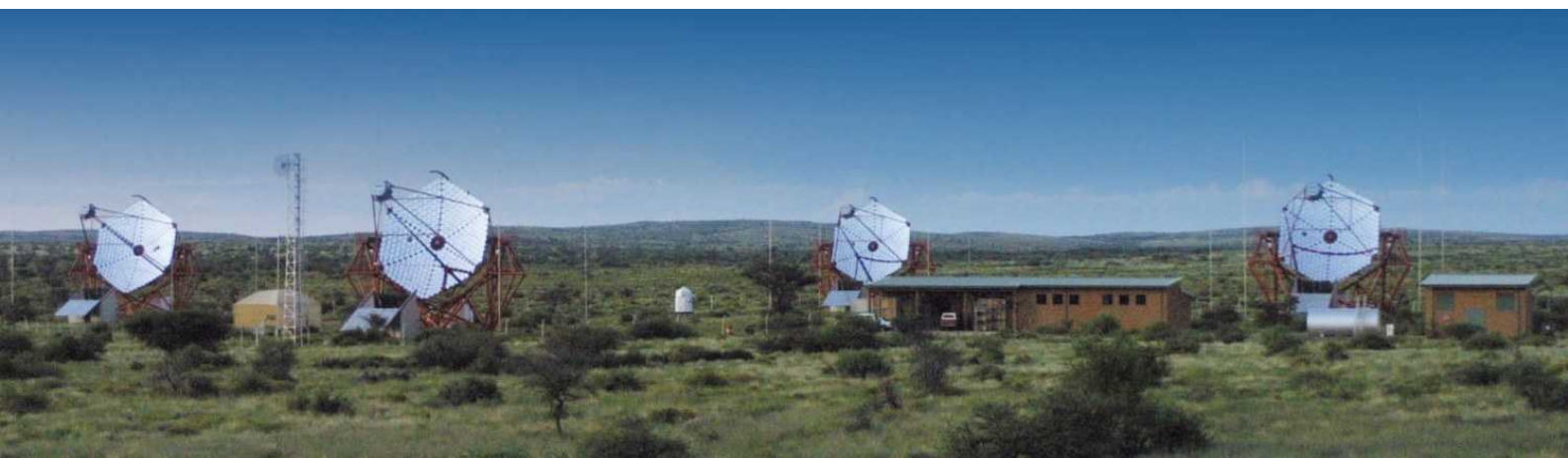
H.E.S.S. Telescopes : The four identical telescopes of the High Energy Stereoscopic System in Namibia detect faint atmospheric flashes caused by the absorption of ultrahigh-energy gamma rays. Credit: H.E.S.S
