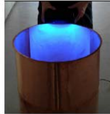
copper shroud lined with reflecting TPB coated Tetratex
