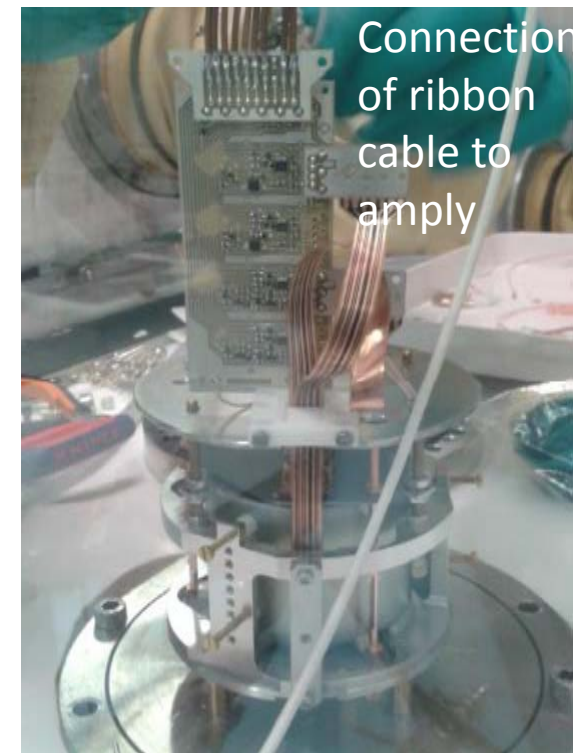
flex cables with JFET and feedback resistor/capacitor
