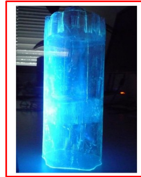
nylon mini-shroud coated with TPB/PS
