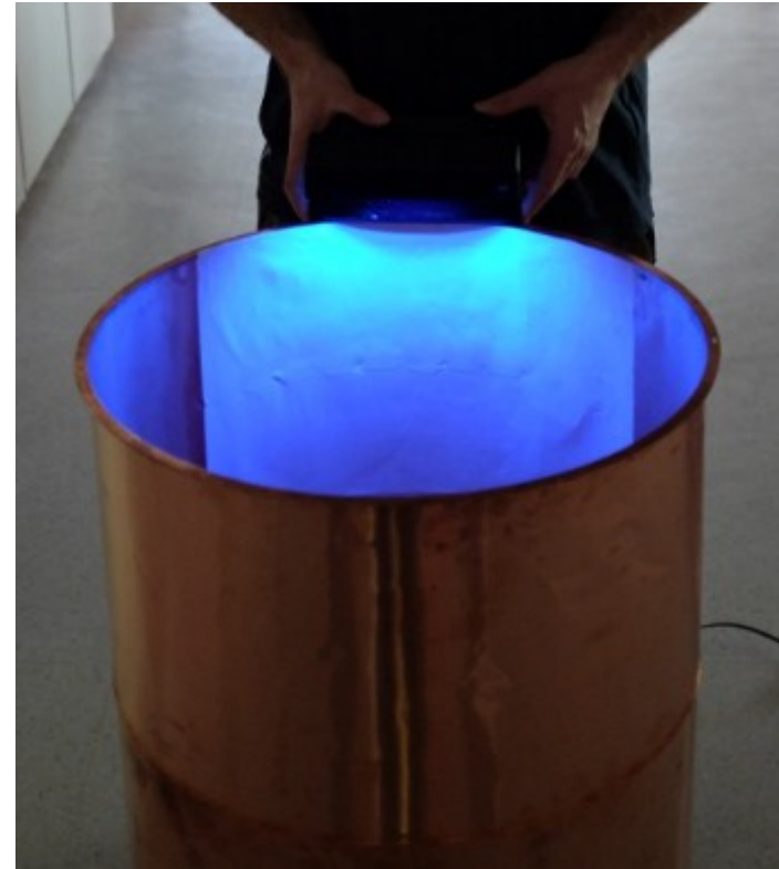
Ø 49 cm - h = 60 cm t = 100 µm copper foil t = 2 mm copper flanges, laser welded
