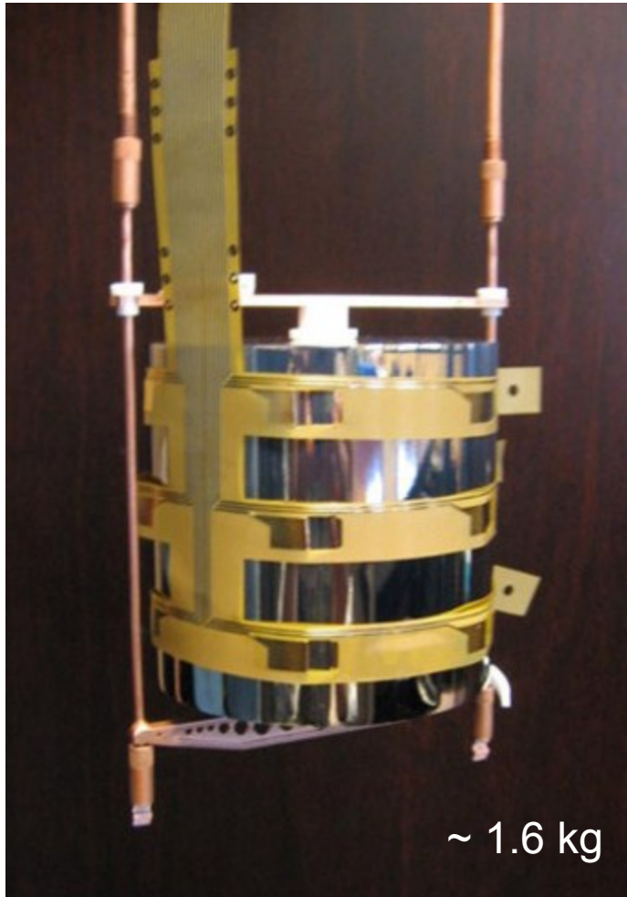
18-fold segmented true coaxial n-type Ge detector
