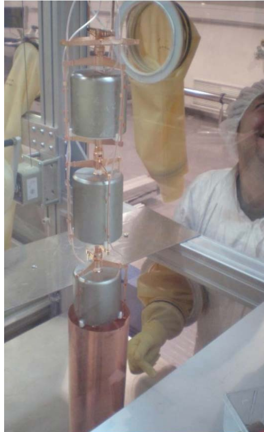
65 \mu\text{m} Cu cylinder ("mini-shroud to Shield E-field")
