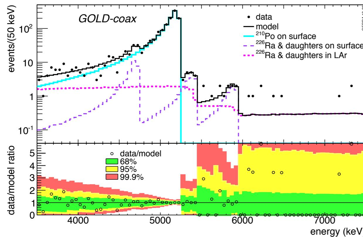
spectral fit with simulated spectra
