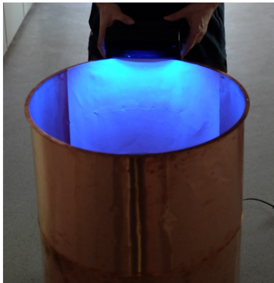
Copper "shroud" with Tetratex reflector coated with TPB
