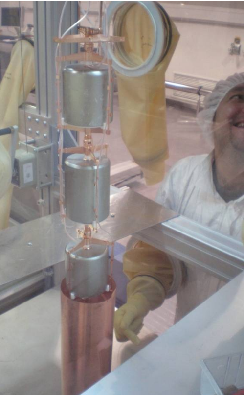
60 \mu\text{m} Cu cylinder ('mini-shroud') to shield E-field
