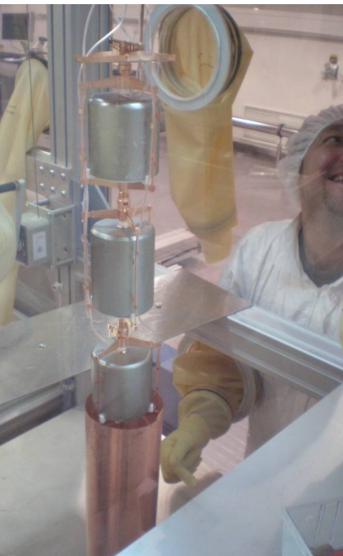
60 \mu\text{m} Cu cylinder ('mini-shroud') to shield E-field
