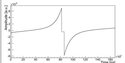
Final filter used to estimate the energy, result of convolution of zero-area finite length cusp filter with the deconvolution filter.
