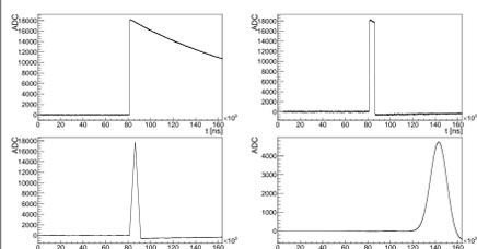
The GERDA signal reconstruction: a digitized waveform (top left), the same after the differentiation (top right) and after applying the MA once (bottom left) and 25 times (bottom right).
