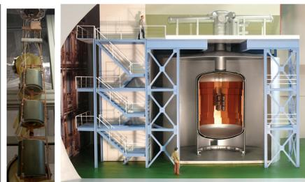
A string with three germanium detectors as they are used in GERDA (left) and a mock-up of the whole experiment (right): the detectors are in a LAr filled cryostat and shielded by a copper layer and a water Cherenkov active muon veto.
