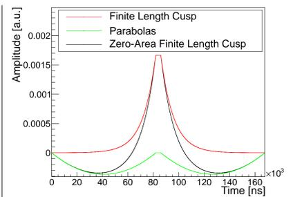
Construction of the zero-area finite length cusp filter (black) as the sum of a finite length cusp filter (red) and two negative parabolas (green).
