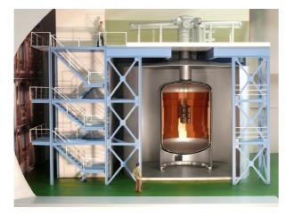
This model of the GERDA experiment shows the onion-like structure which suppresses interfering signals from the environment. The germanium diodes in the center of the cryostat filled with liquid argon (–186°C) are to a larger scale. (©MPI for Nuclear Physics)
