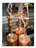
Germanium detectors wrapped by a high-purity copper foil for radiation shielding. (© GERDA collaboration)
