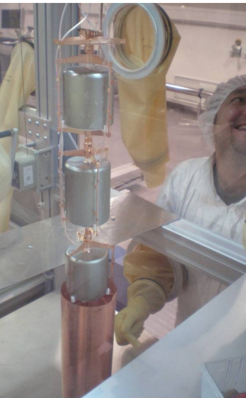
65µm Cu cylinder ('mini-shroud') to shield E-field
