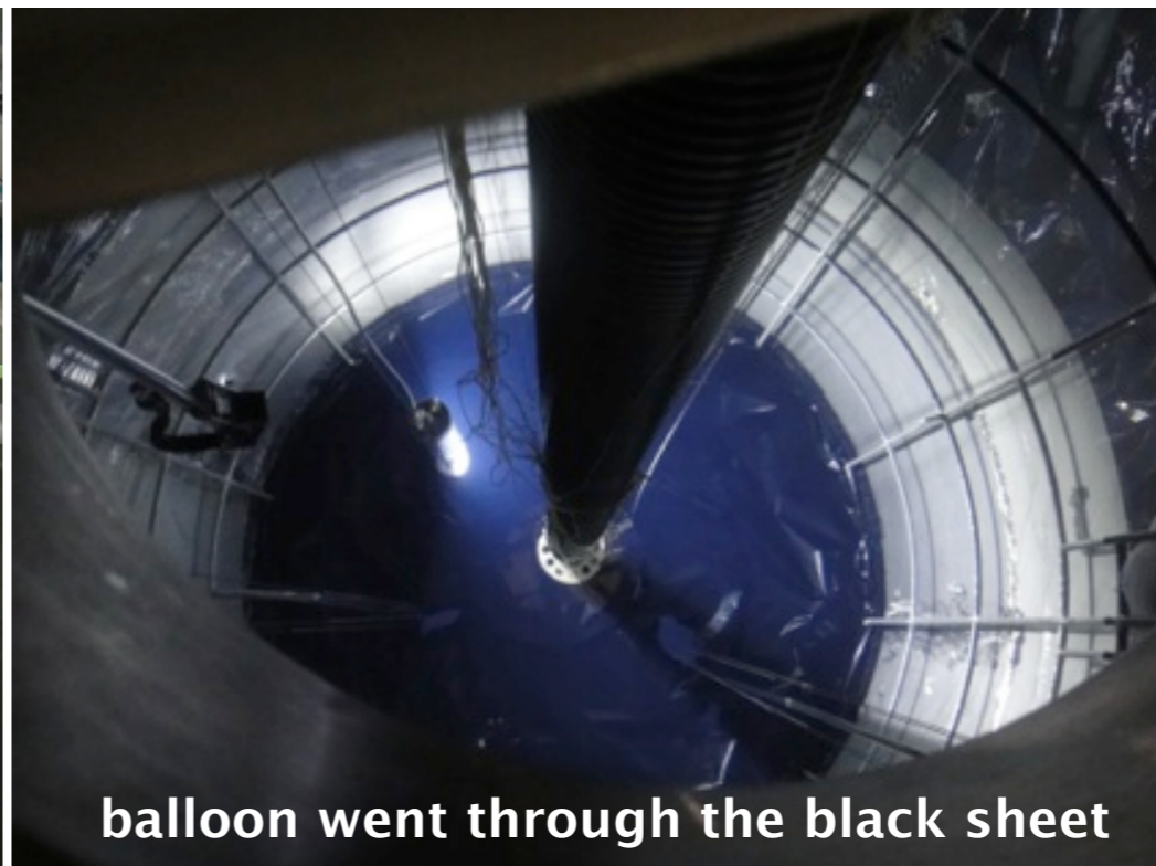
balloon and corrugated tube deployment
