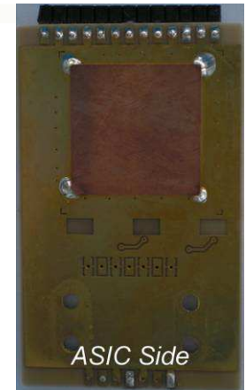
ASIC single-ended preamplifier produced in 0.8 \mu m 5V CZX CMOS technology
