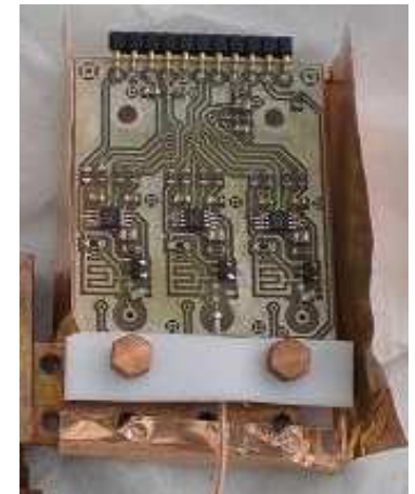
ASIC single-ended preamplifier produced in 0.8 \mu m 5V CZX CMOS technology
