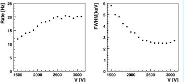
Left: Event rate in the peak of the 1.3 MeV Co-60 line as a function of the applied bias voltage. A stable plateau is reached at 2,500 V when total depletion of the diode is reached. Right: Core energy resolution at 1.3 MeV as a function of the applied bias voltage. Again, a stable (minimal) plateau is reached at 2,500 V. For all further measurements, a bias voltage of 3,000 V was applied.
