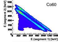
Left: Co-60 spectrum taken with a 6-fold segmented p-type germanium detector submerged into liquid nitrogen. Shown is the energy measured in segment 2 vs. segment 1. A clear correlation for the 1.1 MeV and 1.3 MeV lines can be seen between the segments. This is due to photons which deposit their full energy inside the two segments.
