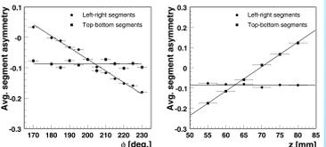
If energy is deposited in a segment mirror charges are induced in the neighboring segments. The asymmetry between the left-right and top-bottom segments are shown for a central segment as a function of the angle  $\phi$  (left) and the height  $z$  (right) using the 122 keV line of Eu-152. A clear correlation between the location of energy deposition and the asymmetry is observed.
