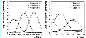
A collimated Eu-152 source was used to measure the segment borders of the detector. The average count rate of the 122 keV line is shown as a function of the angle  $\phi$  (left) and as a function of the height  $z$ . In both cases three segments are clearly visible. The fitted functions are step functions convoluted with Gaussians in order to describe the collimation.
