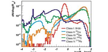
Distribution of the energy spread for different background processes.  $R_{90}$  is defined as the radius which contains 90% of the energy within an event. Class II-IV events have photons in the final state and can be distinguished from Class I and V events which have electrons and alpha-particles in the final state, respectively.
