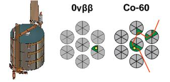
Cross-sectional view onto the GERDA detector array. The signal process has two electrons in the final state which mostly deposit energy in only one segment. In the decay of Co-60 two photons are emitted which scatter and possibly deposit energy in more than one segment. A cut on the segment multiplicity can be used in order to identify events with photons in the final state.
