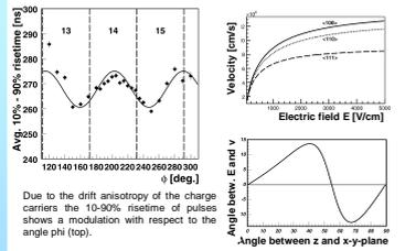
Due to the drift anisotropy of the charge carriers the 10-90% rise time of pulses shows a modulation with respect to the angle  $\phi$  (top). Angle between  $z$  and  $x$ -y-plane.
