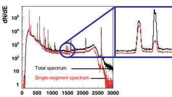
Spectrum measured with a Th-228 source. The black spectrum represents all events whereas the red spectrum represents events with only one segment hit. The close-up shows two peaks. On the left is the double escape peak of the Th-208 line, right is a photon line of the Bi-212. Events in the double escape peak deposit energy locally whereas events in the Bi-212 peak deposit energy over a larger volume and therefore stronger suppressed.
