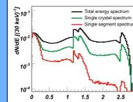
Background rejection due to crystal and segment anti-coincidence for  $^{60}\text{Co}$  in germanium
