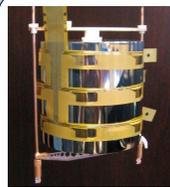
Designed a suspension system such that a minimum of material is used  $\rightarrow$  under test
