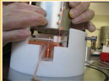
Crystal mounted in the detector holder with HV and signal contacts
