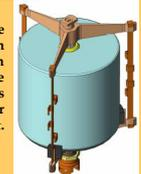
Detector assembly attached to the flange and suspension system in the radon-free clean bench
