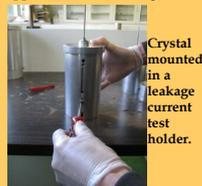
Crystal mounted in a leakage current test holder.
