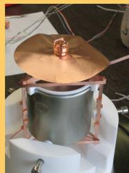
Detector assembly with copper infrared shielding.
