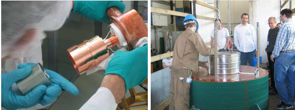
Fig. 3. Left: Dismounting of first enriched detector of the HdMo experiment from its copper vacuum-cryostat. Right: Unloading of the 35 kg enriched germanium. The green cylinder was built to shield the material against cosmogenic activation while transport from Siberia to Germany.
