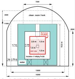
Cross section of the hall A of the Gran Sasso laboratory and a possible tank design with a conventional shield (water/lead) and a cryogenic liquid shield (LN/LAr). This design requires a low <sup>215</sup>Th contamination of the insulation.
