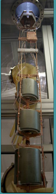
Test stand – detector immersed in cryoliquid
