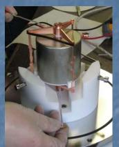
Forward resistivity measurement while cooling
