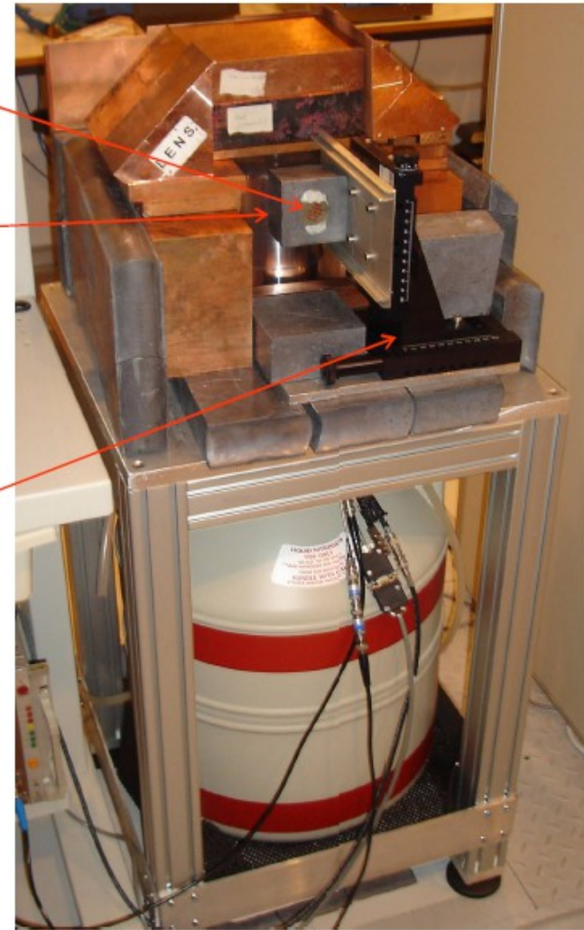
Figure II-14 Left: The geometry of collimator scanning measurements with a ^{241}\text{Am} source, configured for a top surface scan. The collimator with \varnothing 1.5 mm hole is mounted on a precision positioning device allowing movement along the horizontal axis. Right: A photo of the collimator scanning setup configured for a side surface scan. A lead and copper shielding was built around the detector to reduce external background.
