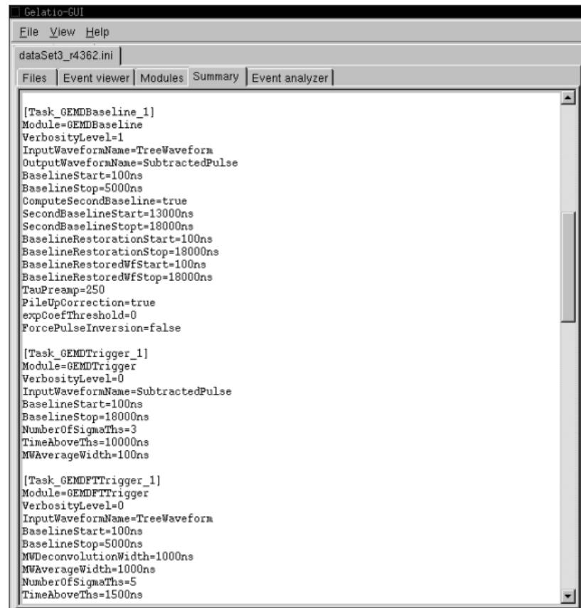
The screenshot shows a window titled "Gelatio-GUI" with a menu bar containing "File", "View", and "Help". Below the menu is a tab bar with "Files", "Event viewer", "Modules", "Summary", and "Event analyzer". The main area displays an ASCII configuration file named "dataSet3\_r4362.ini". The file contains several sections of parameters for different modules:
