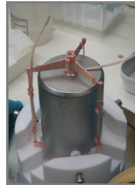
Low-mass holder and electrical contacts
