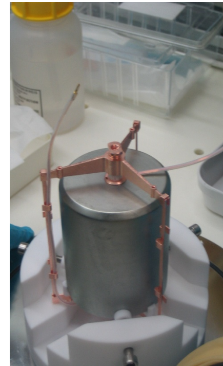
Low-mass holder and electrical contacts
