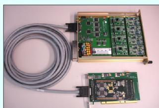
The DAQ NIM module (analog front-end and ADC boards visible on the right) is connected to the PCI receiver board by LVDS signals through commercially available twisted cables.
