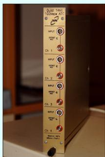
The 4-channels DAQ NIM module, showing differential and single ended input connectors.
