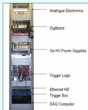
The whole DAQ system (16 channels) for the Germanium detectors of the GERDA experiment at the LNGS underground facility. Additional electronics modules are also present.
