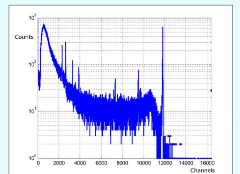
By applying a standard trapezoidal filter, 40  $\mu$ s long with 1  $\mu$ s flat top and no additional baseline subtraction, energy resolution of 4.5 keV FWHM has been achieved for the Thorium spectral line of 2.6 MeV. The available dynamic ranges of the charge sensitive preamplifier and DAQ system were nonetheless above 12 MeV. The digital trigger can then work over a dynamic range of at least a factor of 100, even in presence of picked-up disturbances.
