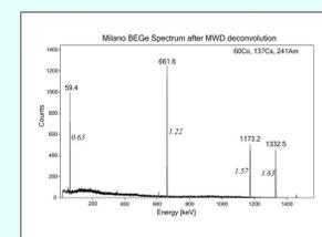
Energy spectrum obtained with the DAQ in auto-triggering mode (1500 events/s), showing the energy resolution (FWHM) for various energy emission lines.
