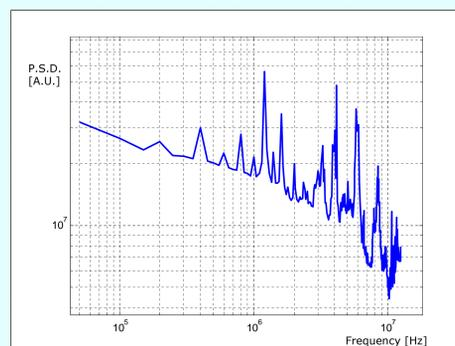
The power spectral density of noise, calculated over the baseline portion of a set of 20.000 pulses, clearly confirms the presence of high-frequency, narrow-banded disturbances, appearing as sinusoidal shapes in time.
