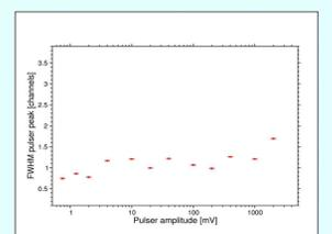
Results of the DAQ linearity test with the pulser, showing non-linearity errors within 1 channel over 16000.
