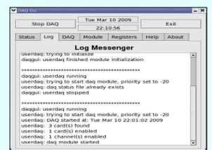
A sample view of the graphical user interface implemented on the PC in order to control the acquisition.
