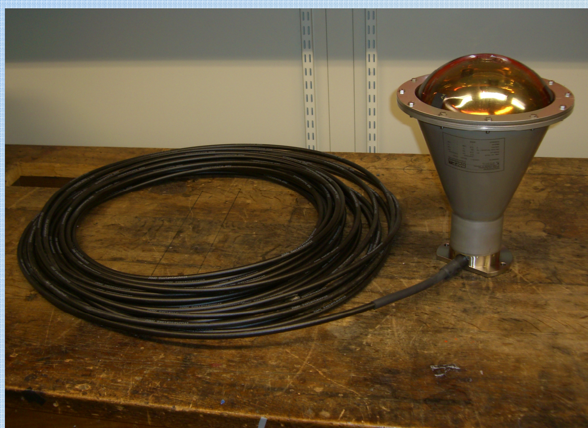
Finished capsule with 32 m cable (RG 213 U)
