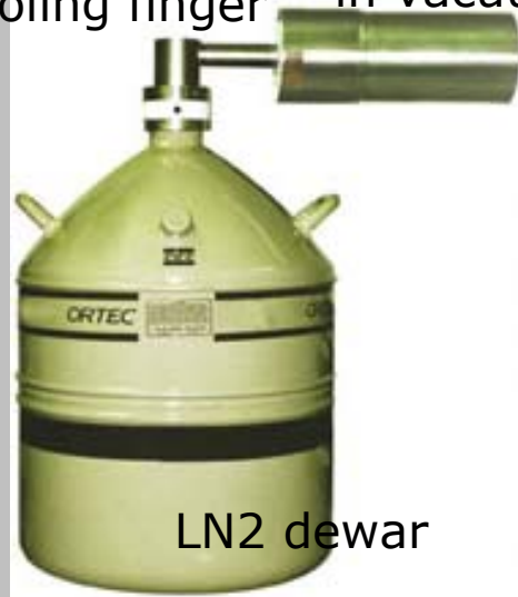
detector cooling finger in vacuum
