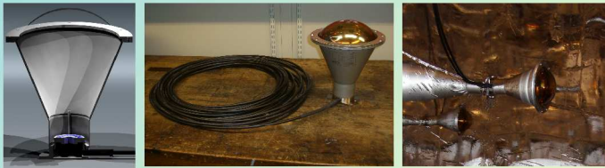
Left: Sketch of the GERDA Photomultiplier capsule Middle: Finished capsule with 32 m cable (RG 213 U) Right: Mounted capsule on the wall of the water tank
