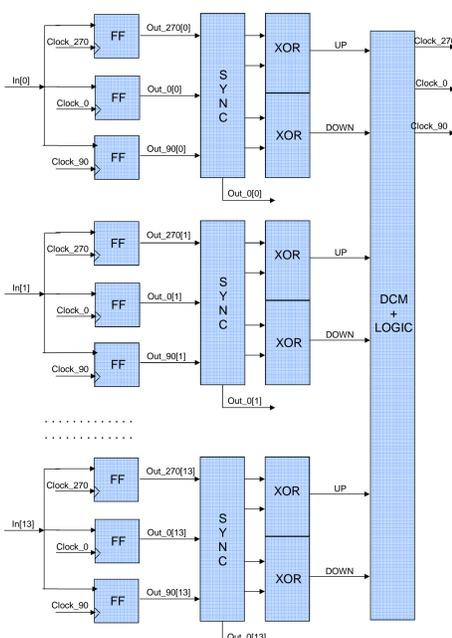
In order to reliably operate ADC signals readout we implemented a real-time self adjusting method to optimally adjust the phase relationship of the ADC readout clock signal with respect to the main system clock (100 MHz).
