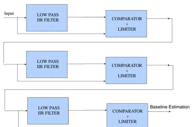
Baseline estimation is based on a recursive procedure, that is implemented by means of resource sharing techniques in FPGA (e.g. a unique high speed block is multiplexed to many low frequency signals).
