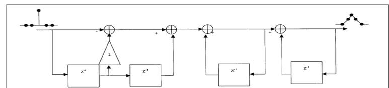
Resource saving implementation in a very tiny Field Programmable Gate Array (FPGA) device (Xilinx Spartan3 50), using Dual Port Block-RAMs and accumulators. The peaking time of the trigger filter is set to 1 us, as a good compromise between signal sensitivity/noise rejection and the ability to detect consecutive events close in time, but could be extended up to about 10 us. (See A. Geraci et al.: "Digital spectroscopy in programmable logic", TNS, IEEE)
