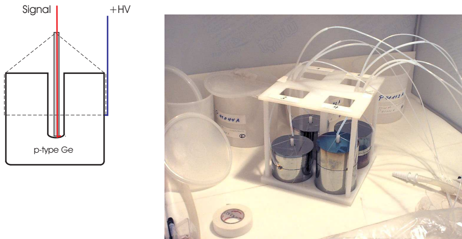
Figure 5.1: The HV and signal cables are connected on the side and central contacts of the diodes, respectively (left). The four first GENIUS-TF bare diodes mounted in the PTFE detector holder (right) [52].
