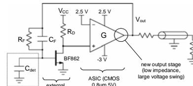
The discrete devices as well as the integrated circuit are mounted on a PCB (Printed Circuit Board) of 0.8 mm PTFE (Teflon) laminate. The ASIC has been realized in a mature CMOS CXZ 0.8 μm 5V technology provided by Austria Micro Systems. The area occupancy of the ASIC is as little as 366x275 μm<sup>2</sup> excluding the bonding pads.
