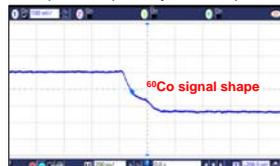
Preamplifier output signal as acquired in a longer time scale when a <sup>60</sup>Co radioactive source is irradiating the detector.
