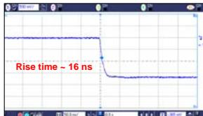
Leading edge of a typical signal from a <sup>60</sup>Co source. The preamplifier wide bandwidth permits use of pulse-shape analysis techniques.
